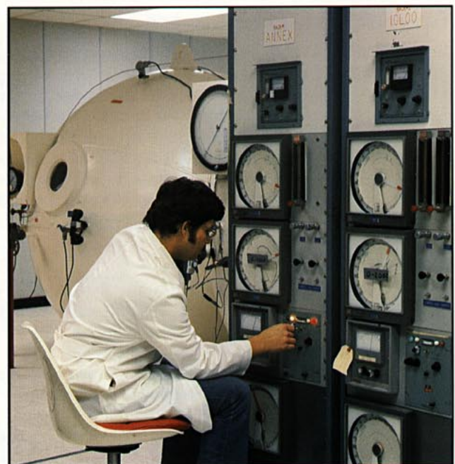
The oxygen content of the breathing mixtures in this large hyperbaric diving chamber is monitored by a percent oxygen analyzer. The chamber, used for diving research and training, can simulate pressures equivalent to depths of 2200 feet.
